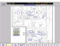
QSPEC Solutions' client is confidential life sciences manufacturer. The purpose of the Environmental Monitoring System is provide regulatory required monitoring of the air quality pressures (differential and particulate counts) in the production areas of the pharmaceutical plant. This project involved replacing the existing overloaded and unreliable Opto-22/PC based system with a PLC based SCADA system.
